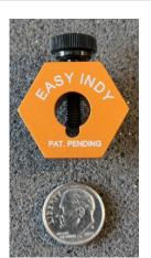
The **SMALL** "EASY INDY" is designed to work in most all Swiss machines and small lathe machines that use 3-pronged style collets. The 3-prong thickness of this tool is .040/.050 wide. It will not fit in some style collets with an extremely wide slot, example LT12 12mm collet. The tool is designed to accept the indicator alone (small hole) or any length extension. This tool is not designed or made to insert or remove collets.
