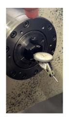
The **MEDIUM** "EASY INDY" is designed for fast and easy precision tool indication, in small to medium size lathes. It will fit most all 3-sided or 3-pronged collets and collet pads. s22 pads, s16 pads, 5c collet, dead length collets and many more. The three tabs on the 'EASY INDY" indicator holder measure .06 - .100 thick. The newer version will fit pads and collets.
