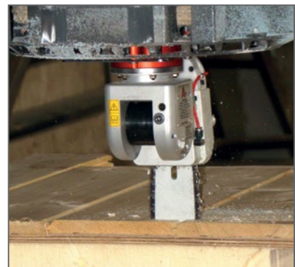
Cutting pocket with chainsaw
