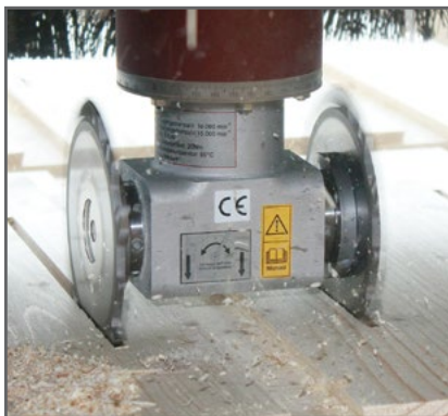
Dual sawing operations
