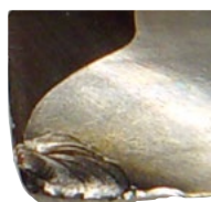
ER chuck wear detail
