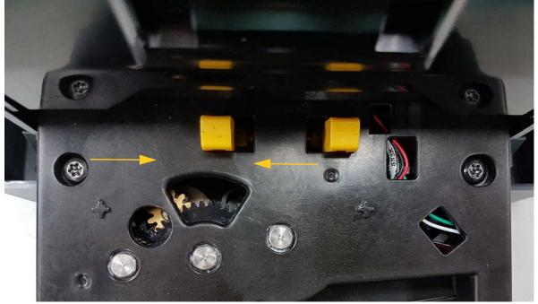
3. Rotate the cutter gear counter-clockwise to lower the blade.
