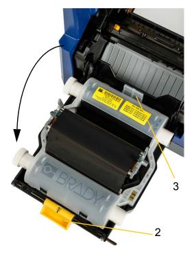
4. Place ribbon cartridge with ribbon over print head (product label toward machine), then snap into place.
