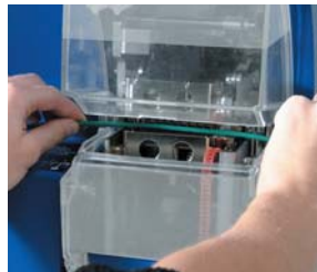
Select job, insert wire or cable.
