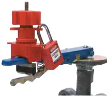
Clamp attaches to butterfly handles, preventing trigger handle from being squeezed. Valve cannot be repositioned!
